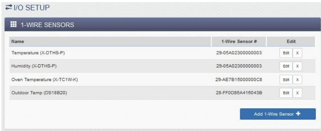
To add a new local 1-Wire sensor, click *Add 1-Wire Sensor* in the local 1-Wire Sensors table.
